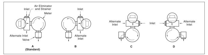
Meters will be set up as indicated by Arrangement "A" unless otherwise specified.
