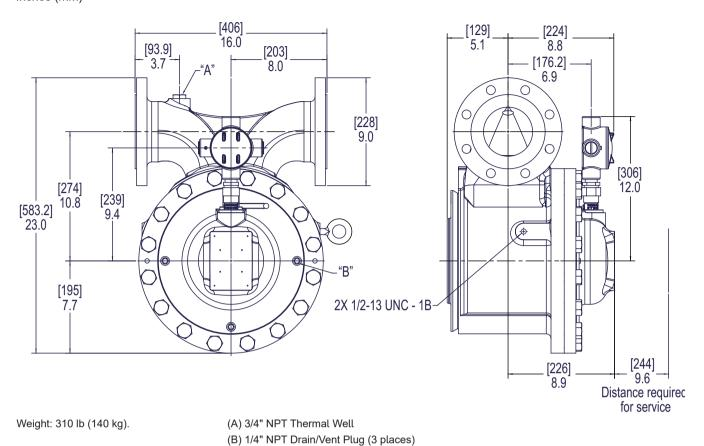
Note: Dimensions – Inches to the nearest tenth (millimeters to the nearest whole mm), each independently dimensioned from respective engineering drawings.
