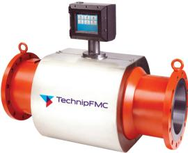
The high speed electronics measure the transit time in both the upstream and downstream direction. This information is used to accurately calculate the flowing velocity and volumetric flow rate of gas through the meter.
