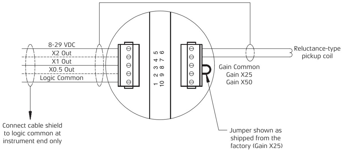
**Note:** In wiring the Reluctance-Type Pickup Coil, the white wire must be connected to Terminal 6 and the black wire to Terminal 7. This is critical when used for dual pulse input to an electronic instrument.
