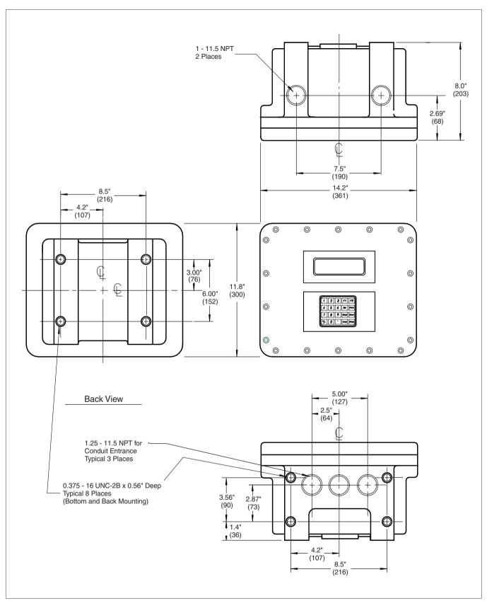
Figure 2 - Explosion-Proof Housing - ALIII-S Hardware
