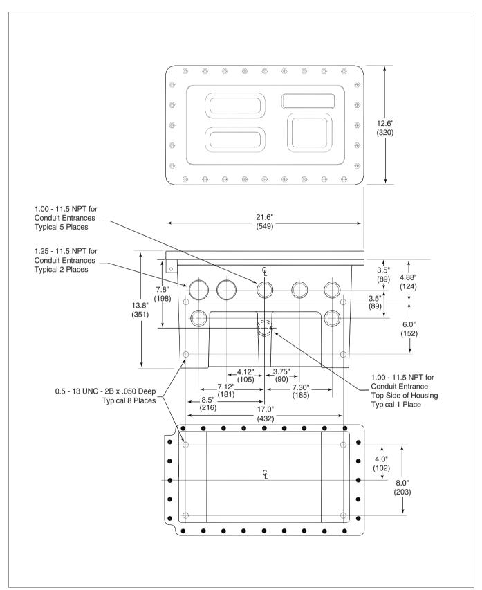
Figure 1 – Explosion-Proof Housing – ALIII-Q Hardware
