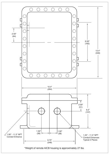
Figure 3 - Remote Housing (Optional AICB)
